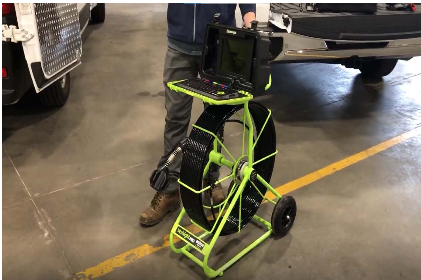
Figure 1 Photo of RIDOT CCTV push camera, new state of the art technology for inspecting small diameter pipes
