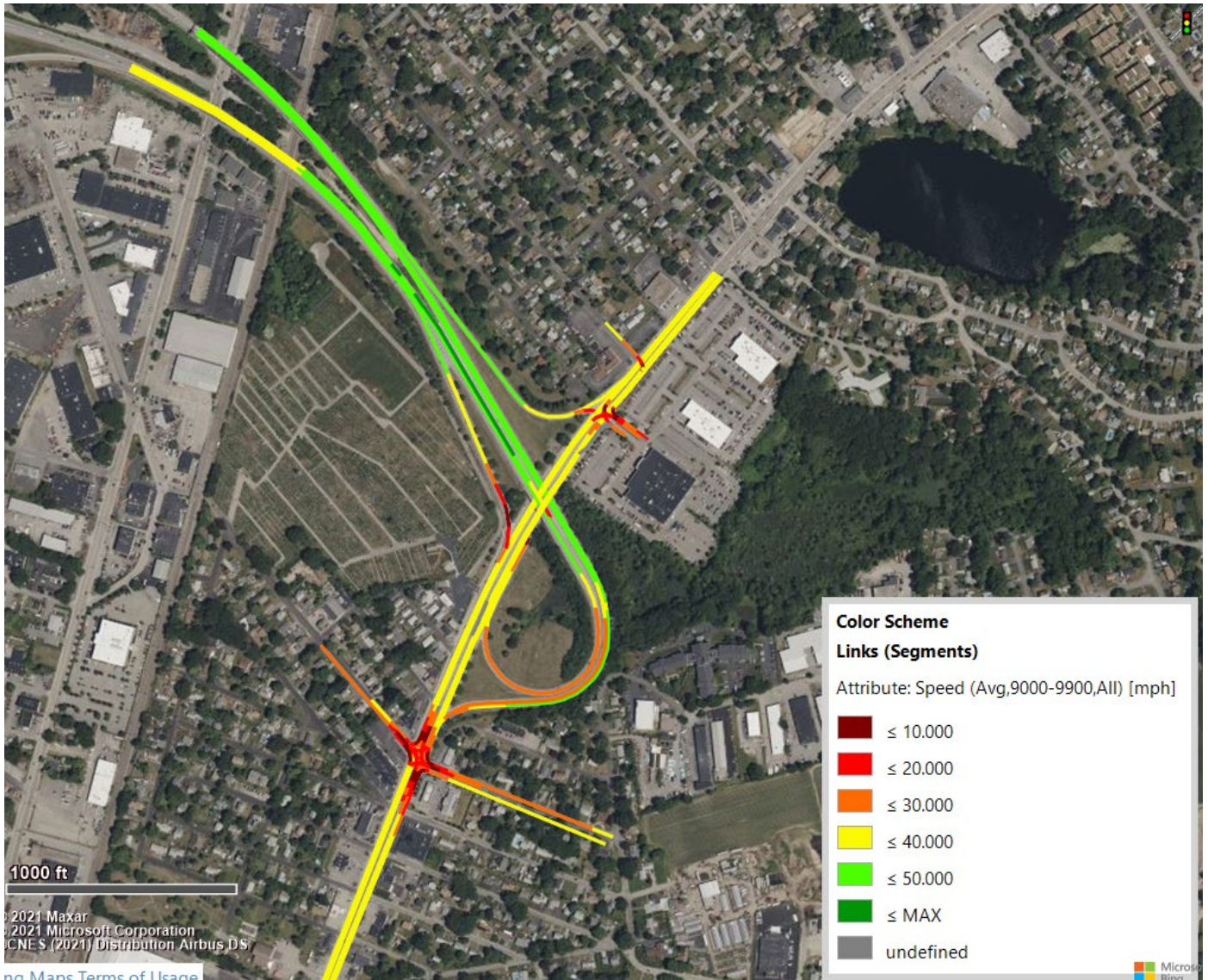
Figure 2 2023 Existing AM Peak Condition
