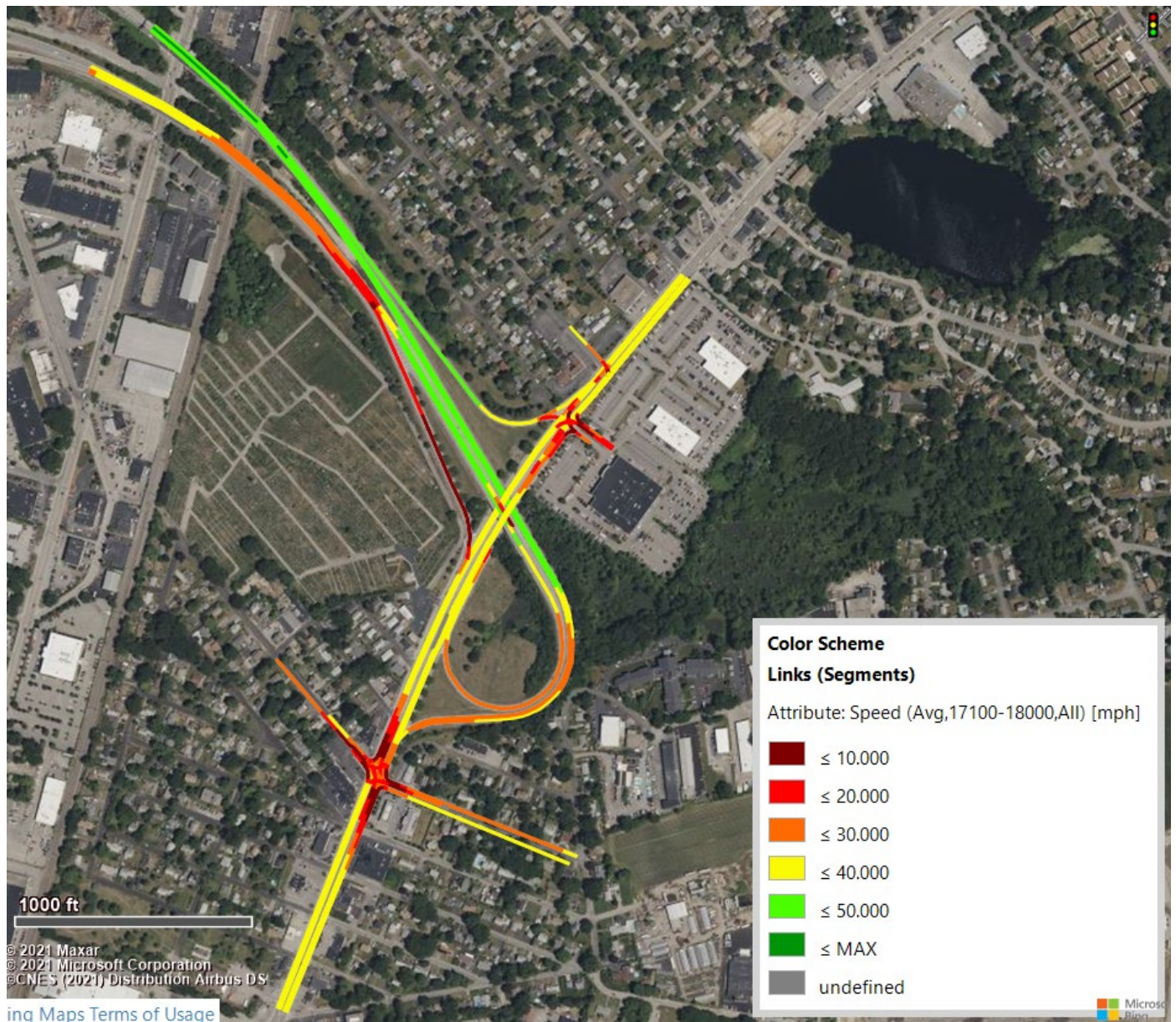
Figure 3 2023 Existing PM Peak Condition
